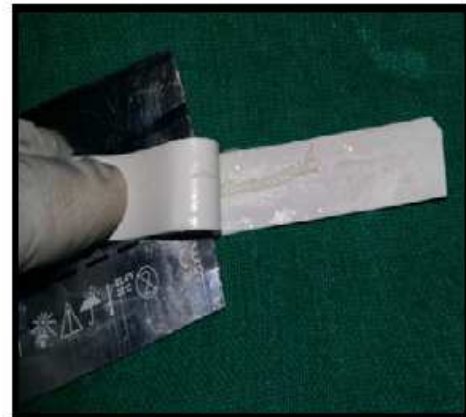
Fig.6. Interlig material used (glass fibre reinforced composite)
