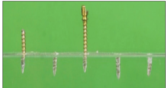
Figure 11. Mini-implants of SK Surgical Showing the Fracture at the Head
