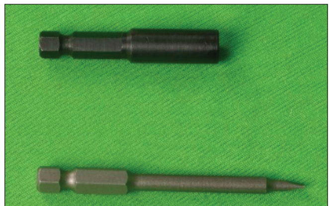
Figure 9. Customized Bits for the Insertion of Mini-implants in the Block
