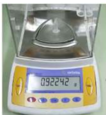
Figure no.8: Analytical Digital weighing balance (Sartorius, Nona Technologies Pvt. Ltd, Bengaluru)
